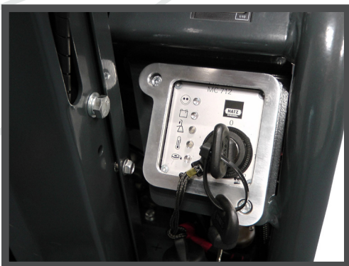
ELECTRIC, KEY IGNITION START & LED WARNING LAMPS (DIESEL ELECTRIC MODEL)
